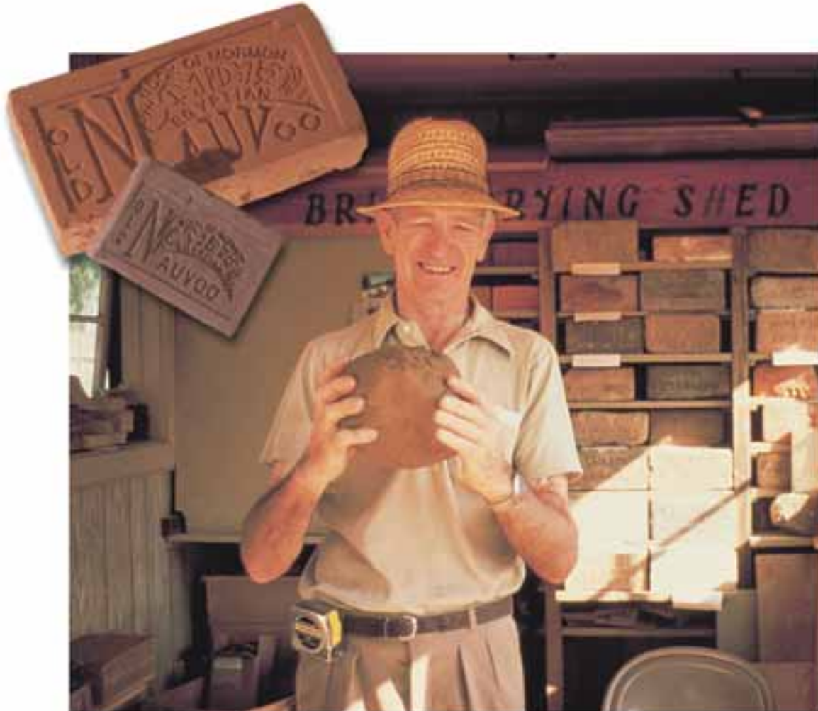
Above: Missionaries Everett and Verna Belcher stand in front of the brick kiln they built in Nauvoo in 1980. Left: Elder Belcher works the clay in his brick-making shed in 1980. He then molds the clay into bricks (below) and stamps a design of his own creation into the bricks before firing them in the kiln (below left). Upper left corner: Finished bricks.
